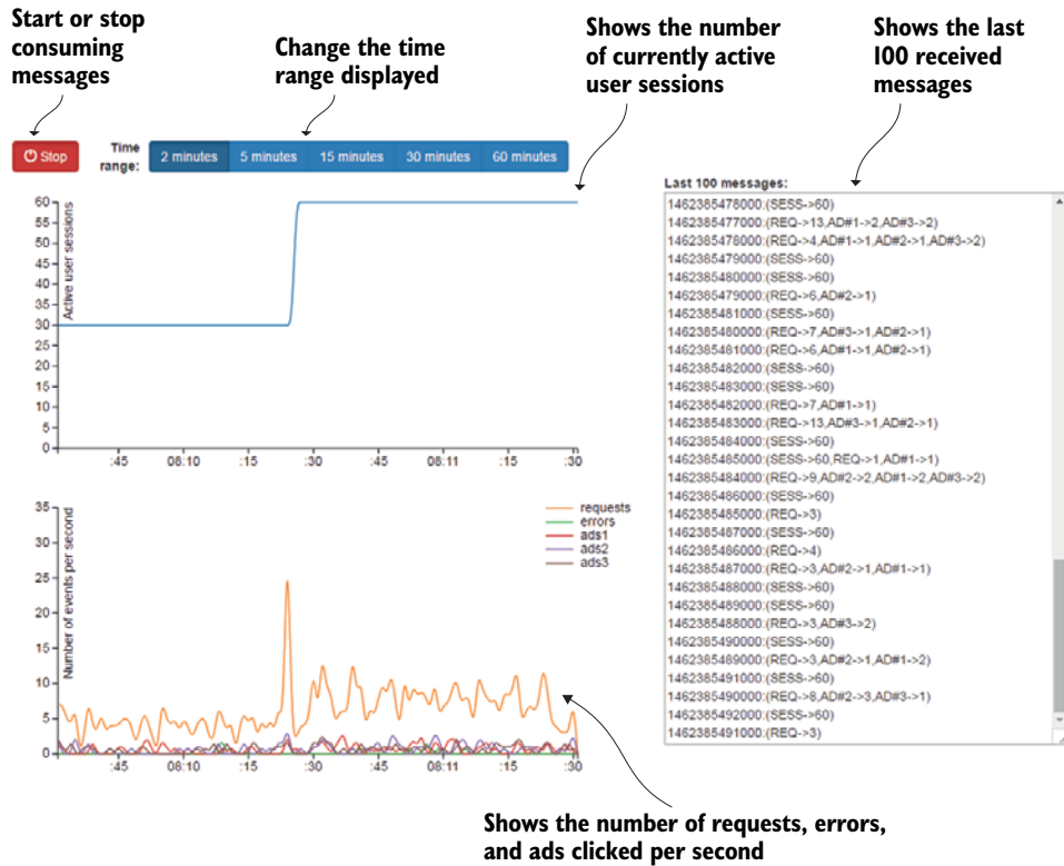
Figure 13.1 Web Stats Dashboard displays two graphs: one showing the number of active user sessions and the other showing the number of requests, errors, and ads clicked per second. You can change the displayed time range using the buttons at the top, and start or stop consuming messages using the button in the upper-left corner. The last 100 messages are shown on the right for debugging purposes.
